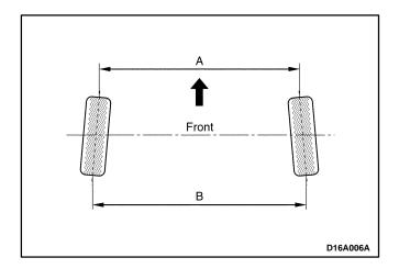
Toe—in is the turning in of the tires, while toe—out is the turning out of the tires from the geometric centerline or thrust line. The toe ensures parallel rolling of the wheels.
