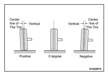
Camber is the tilting of the top of the tire from the vertical when viewed from the front of the vehicle. When the tires tilt outward, the camber is positive. When the tires tilt inward, the camber is negative. The camber angle is measured in degrees from the vertical. Camber influences both directional control and tire wear.
