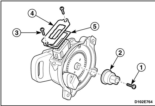
4. Remove the optical sensor cover and adaptor from the distributor housing.
