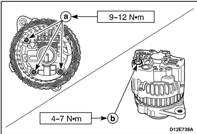
2. Install the bolts / nuts / screws.
