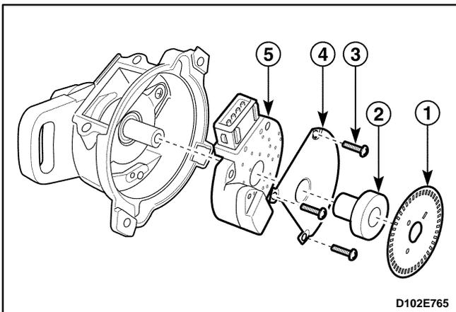
5. Remove the optical sensor unit from the distributor housing.
