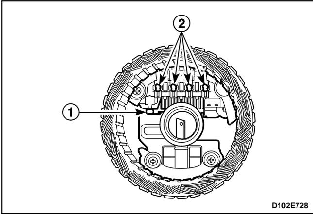
8. Remove the rectifier / brush holder / regulator from the stator.
