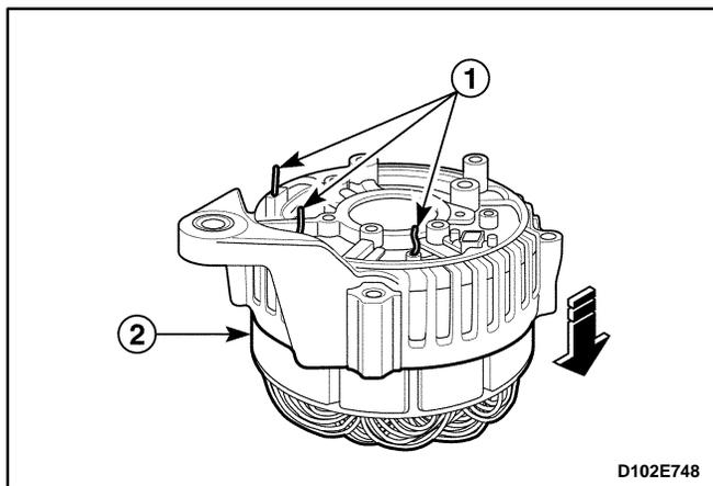
8. Remove the stator assembly from the frame.
