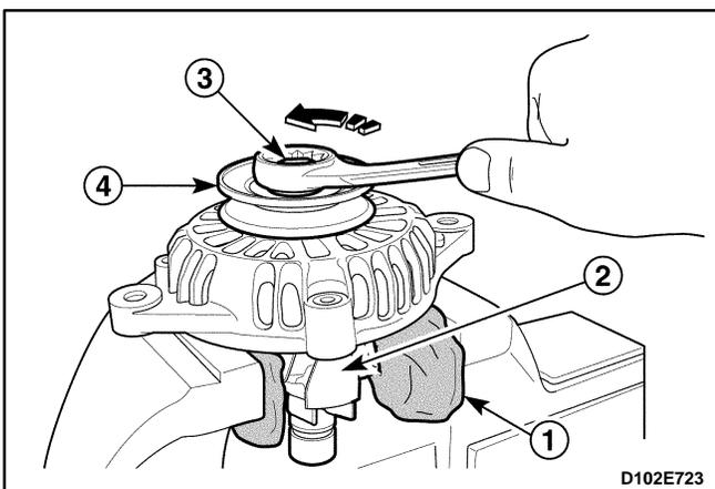
3. Remove the pulley and rotor assembly from the front bracket.
