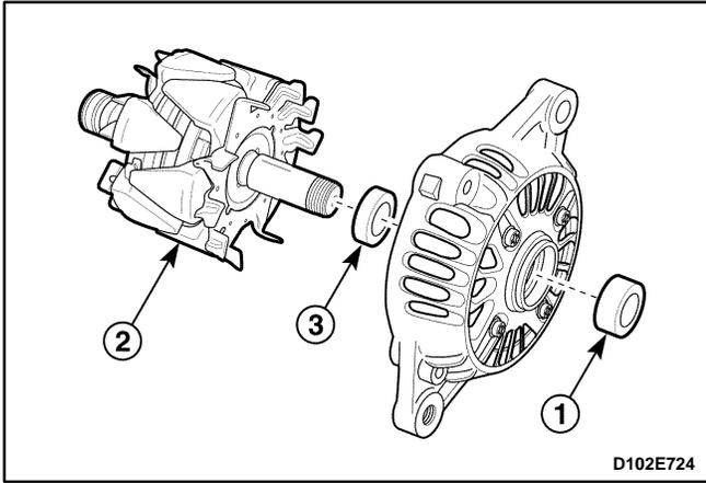
4. Remove the front bracket, rotor and collar.
