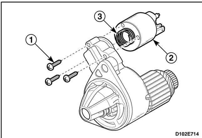
4. Remove the solenoid assembly.
