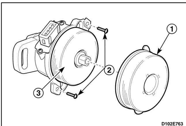
3. Remove the inner / outer cover from the distributor housing.
