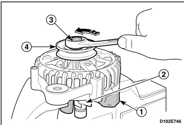
6. Remove the pulley and rotor assembly from the drive end bracket.
