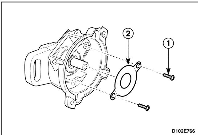
6. Remove the bearing plate from the distributor housing.
