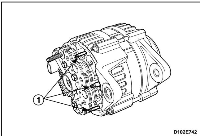
3. Remove the regulator / brush holder / rectifier assembly.
