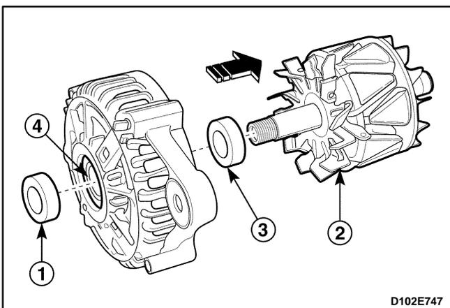
7. Remove the drive end bracket, rotor and space.
