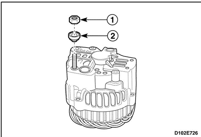
6. Remove the battery positive terminal nut from the rear bracket.
