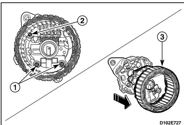
7. Remove the stator assembly from the rear bracket.
