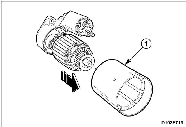
3. Remove the field frame assembly from the armature set (1).
