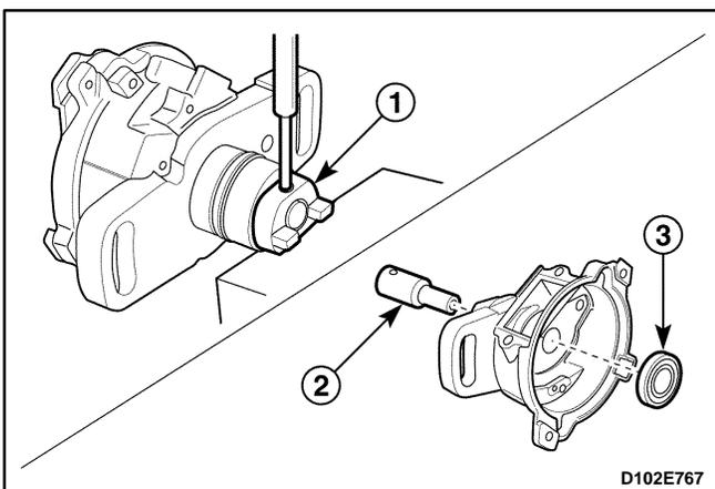
7. Remove the coupling, shaft and bearing from the distributor housing.
