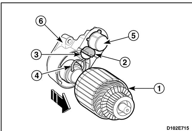
5. Remove the armature set and solenoid from the starter housing.
