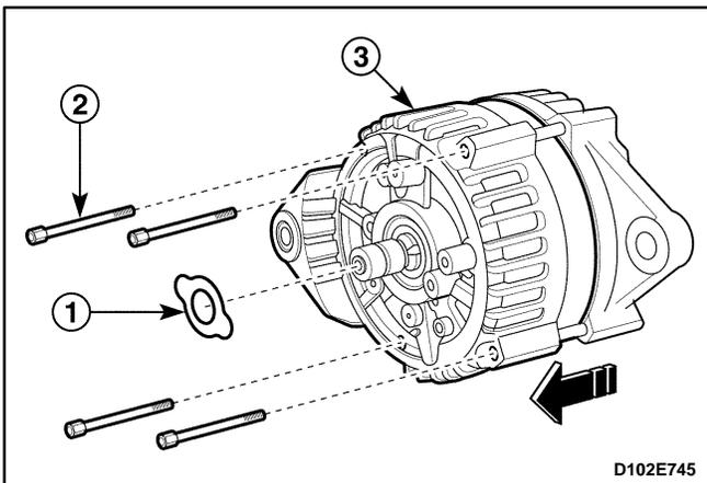
5. Remove the shield before the drive end bracket and the frame.
